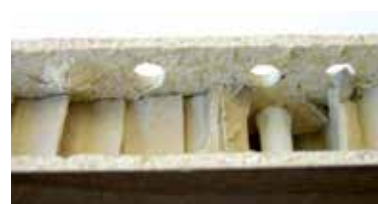
Drill bit comparison left: standard drill bit right: Stehle VHW Dowel Bit
